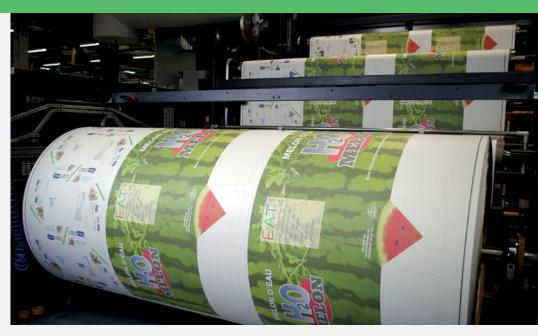
With print speeds up to 305 m (1000 ft) per minute, print with great agility to accelerate turnaround times and lower minimum order quantities requirements that optimize inventories, while focusing analog print capacity on longer runs.
